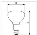
This infrared reflector lamp is designed to operate in the harshest environments such as farms, bathrooms or kitchens and other industrial environments. They have a reinforced construction due to the use of solid glass.
